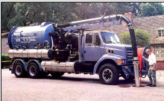
FIGURE 2-3 Catch basin cleaning. SOURCE: Robert Pitt, University of Alabama.
