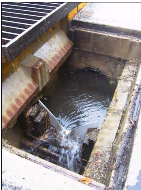
FIGURE 5-54 Weir flow used to measure flow rate. SOURCE: Robert Traver, Villanova University.
