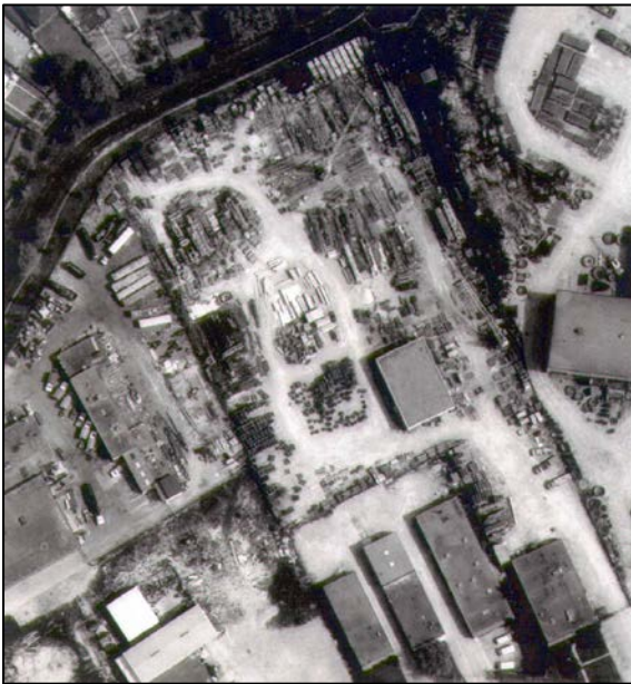
FIGURE 3-4 Example of a high-resolution panchromatic aerial photograph of an industrial area used for measurements of urban surfaces. SOURCE: Pitt and McLean (1986).
