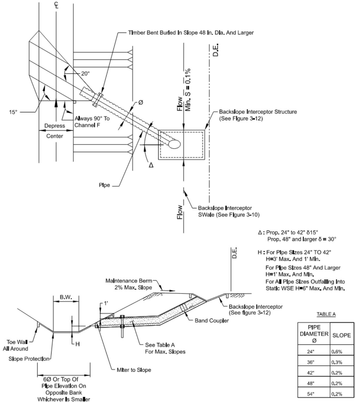
Figure 3-11 Backslope Interceptor Structure
