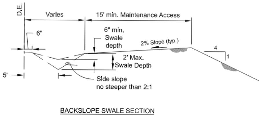
*Figure 3-10 Typical Backslope Drain*
