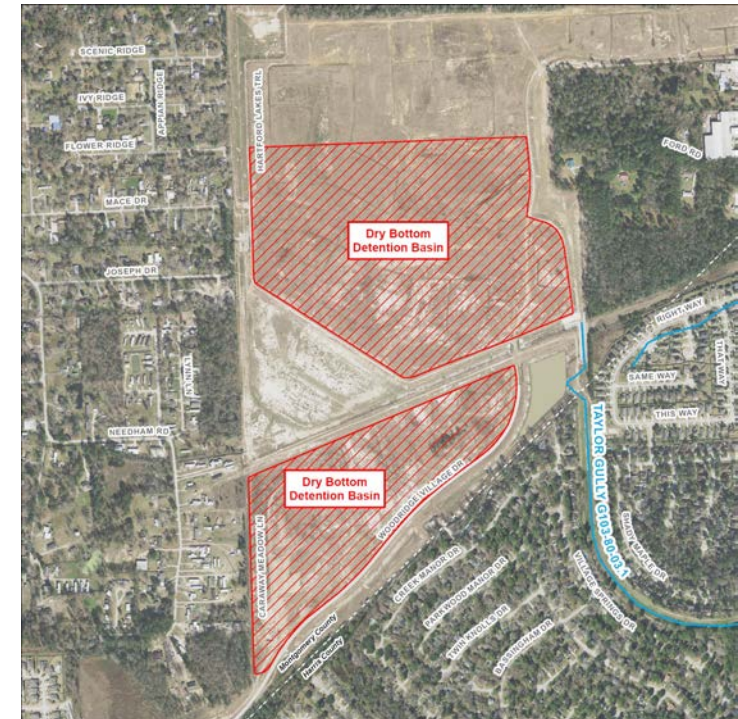
Detailed view of stormwater detention basin site
