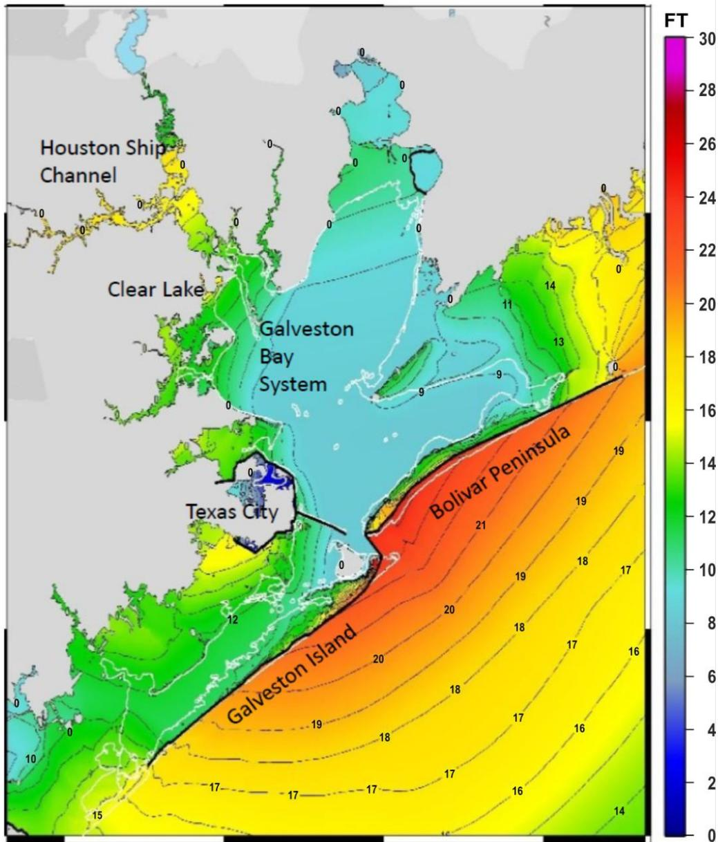
Figure 3. Hurricane surge flooding from a moderate category 3 storm with the characteristics of Hurricane Ike with the coastal spine in place. The Texas City industrial complex is protected by the existing levee, but 12 to 14 feet surge extends inland in the Bayport area and reaches 18 to 20 feet up the Houston Ship Channel. Graphic courtesy of SSPEED Center.
