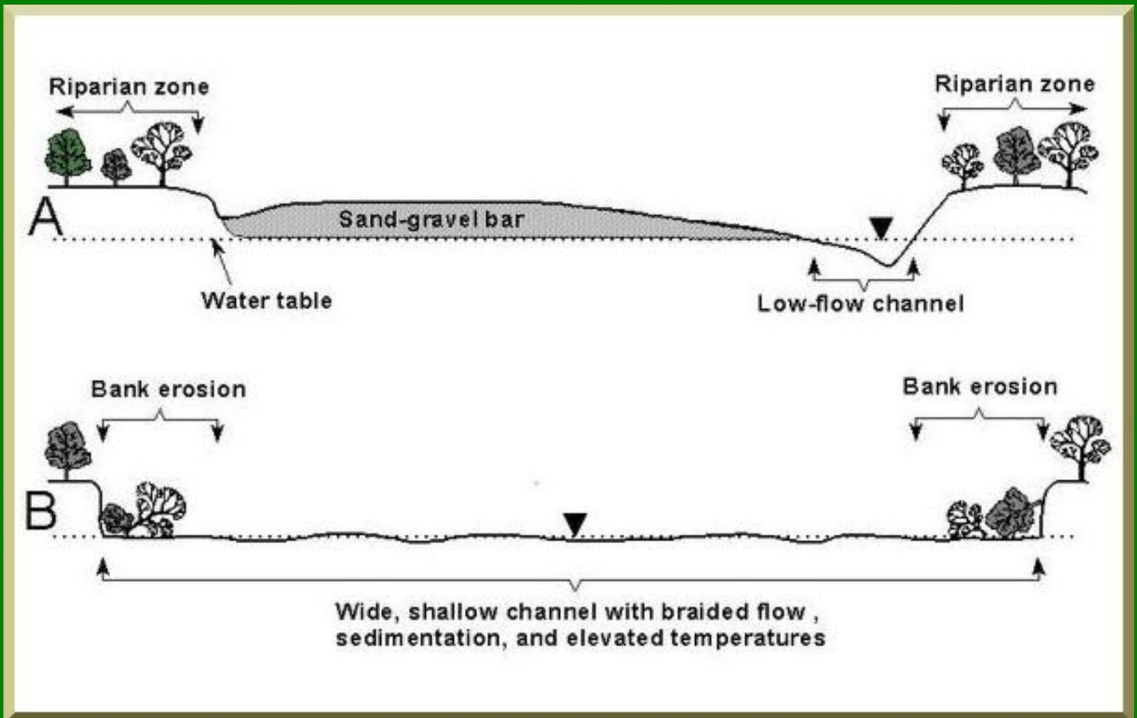
**Fig. 2** Diagram of channel cross sections showing (A) a typical sand-gravel bar in relation to the low-flow channel, riparian zone and water table, and (B) the wide shallow channel that results from unrestricted mining and that is characterized by bank erosion, braided flow, sedimentation, and increased water temperatures.
