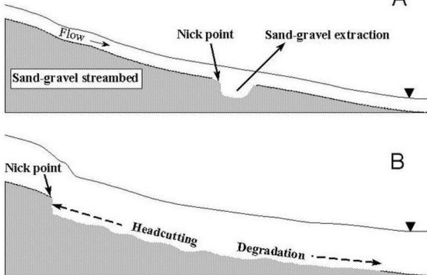
**Fig. 1** Diagram of sand-and-gravel stream bed showing (A) the nick point that develops with a pit excavation, and (B) the upstream head cutting and downstream bed degradation that develop during high flows.
